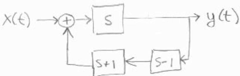
using the standard formula for feedback, write the differential equation for the system above
