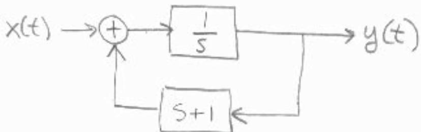
write the differential equation for the system above .
