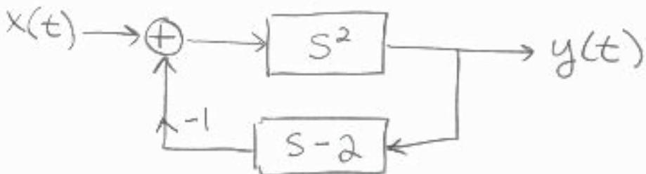
write the differential equation for the above system
