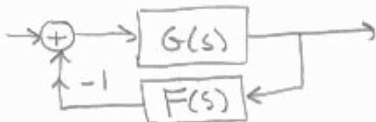
where the differential equation for  $G(s)$  is  $\frac{dy(t)}{dt} = x(t)$  and for  $F(s)$  is  $\frac{dy(t)}{dt} = x(t)$
