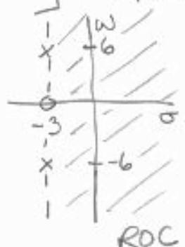
$$\frac{d^2y(t)}{dt^2} + 6\frac{dy(t)}{dt} + 45y(t) = \frac{dx(t)}{dt} + 3x(t) \quad \begin{array}{l} \text{Stable} \\ \text{ROC contains } w\text{-axis} \end{array}$$
