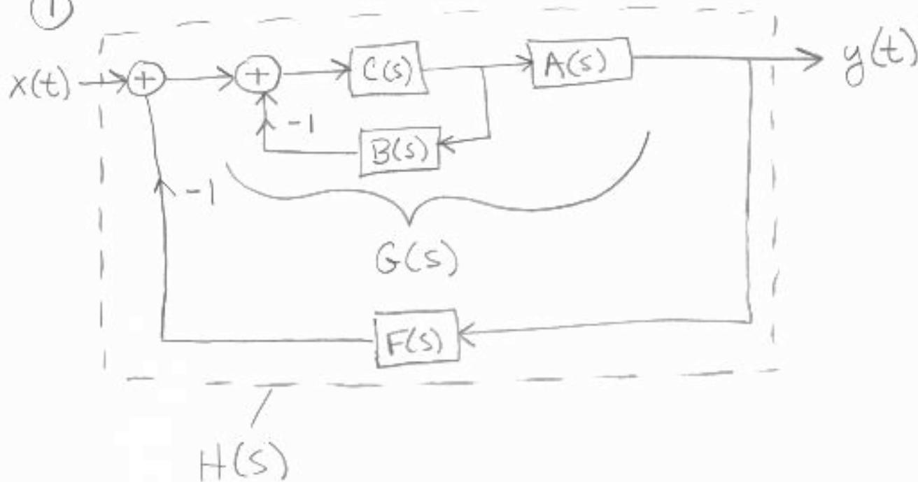
Using the standard formula for Closed loop gain, derive an expression for  $H(s)$  by first finding  $G(s)$ .
