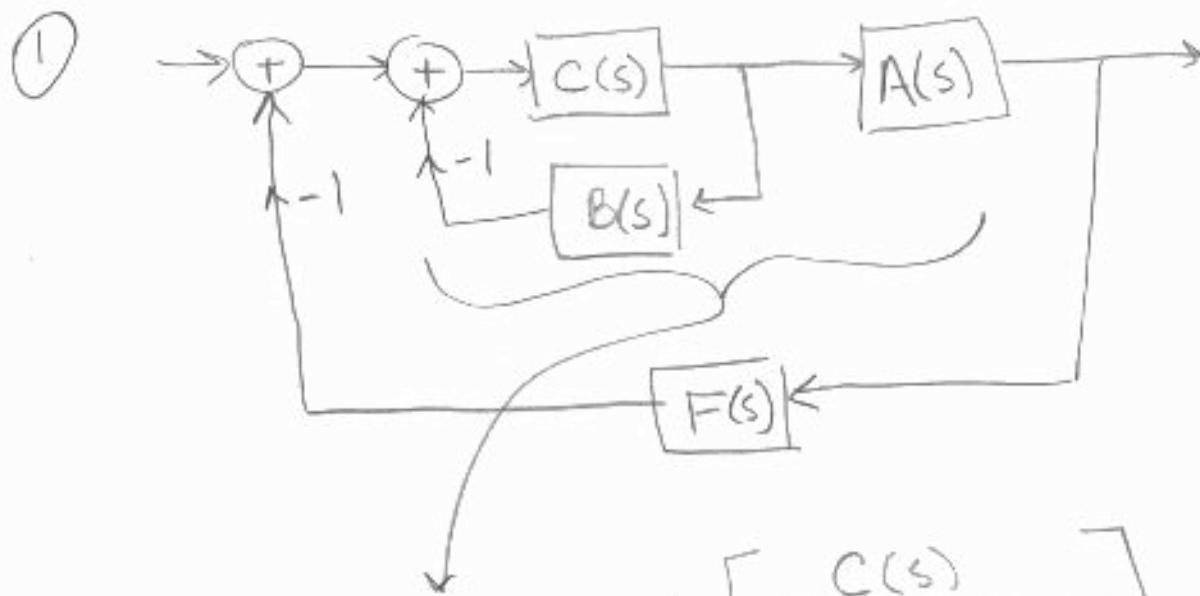
open loop gain  $G(s) = A(s) \left[ \frac{C(s)}{1 + B(s)C(s)} \right]$
