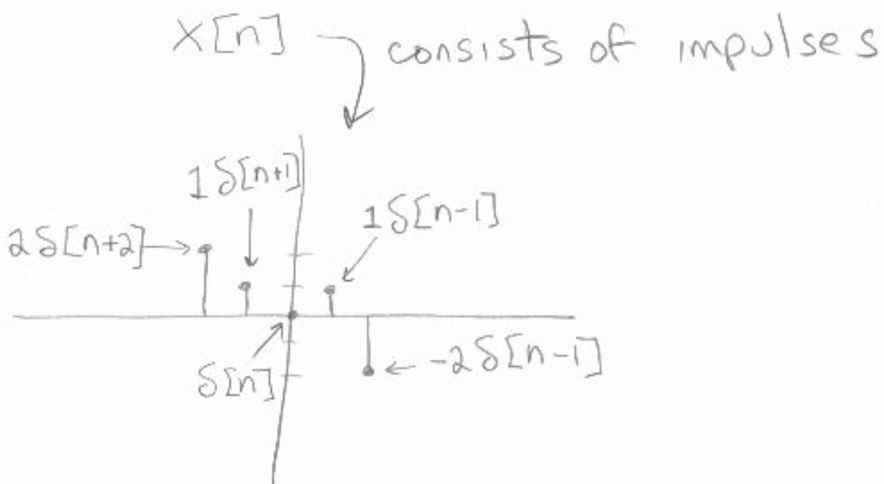
ANY  $x[n]$  can be broken up into scaled and shifted impulse functions.
