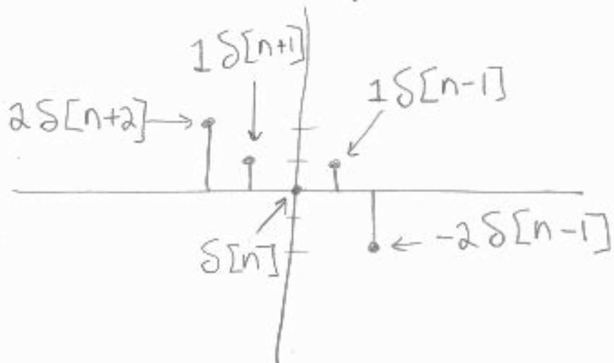
ANY  $x[n]$  can be broken up into scaled and shifted impulse functions.
