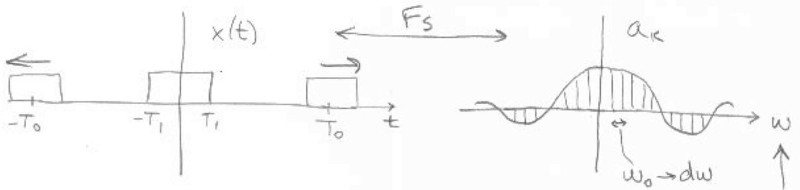
$$\omega_0 = \frac{2\pi}{T_0} \quad \text{as } T_0 \rightarrow \infty, \omega_0 \rightarrow 0$$
