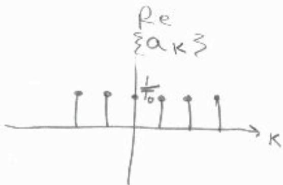
$$a_k = \frac{1}{T_0} \int_{-\frac{T_0}{2}}^{\frac{T_0}{2}} \delta(t) e^{-j k \omega_0 t} dt = \frac{1}{T_0}$$
